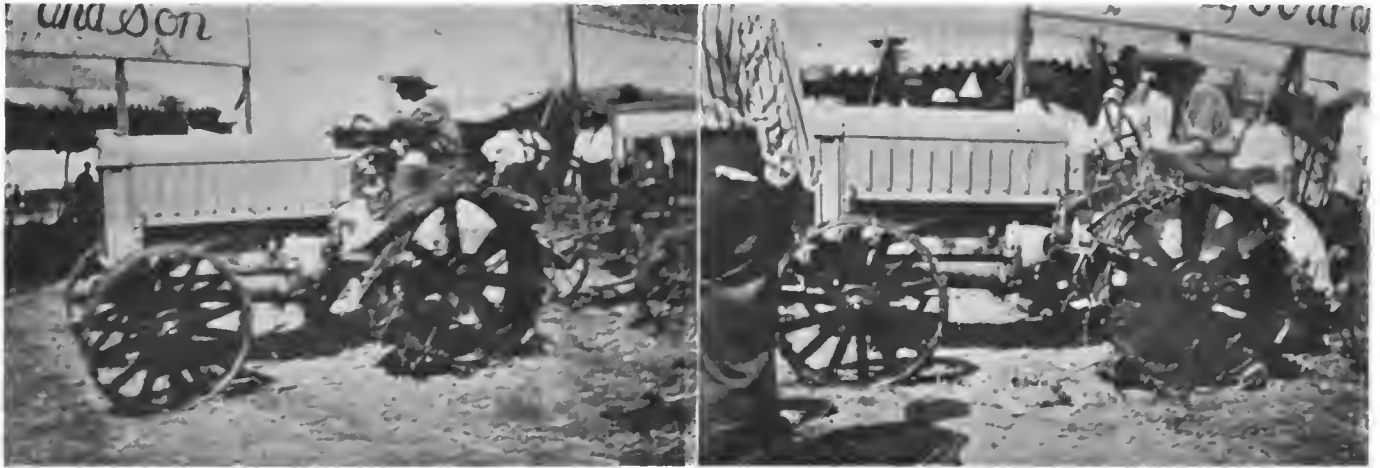
The new Ford tractor at the Fremont, Neb., tractor demonstration. It is a four-wheel design using a four-cylinder motor 4 by 4 1/4, multiple-disc clutch, three-speed and reverse, constant-mesh type of gearbox and worm-drive to the rear axle. It weighs less than a ton. The price has not yet been set. It pulls two plows at a speed of 2 to 2 1/2 m.p.h., and will travel at 5 to 6 m.p.h. on the road.
